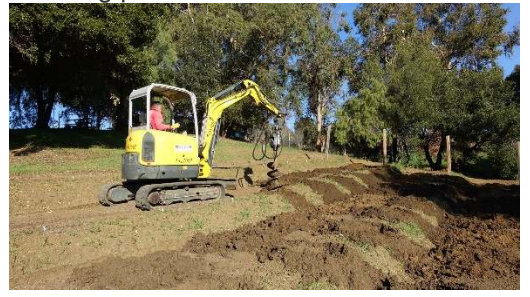
4 Drilling plant holes with an excavator
